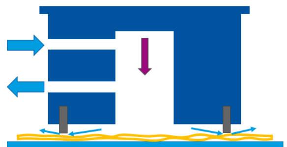
Measuring method roughness acc. Bendtsen
